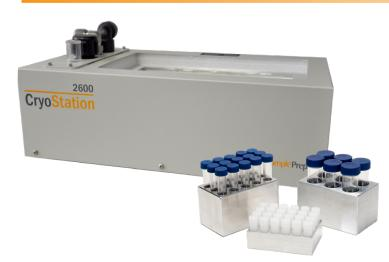
Our Kryo-Tech® Accessories offers a solution for preserving pesticides, RNA or proteins while being ground in the 2010 Geno/Grinder.® Our Cryo-Blocks are designed to be chilled in the 2600 Cryo-Station.
