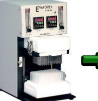
• Inexpensive nitrogen evaporators for plates can rapidly concentrate or evaporate extracts to dryness
