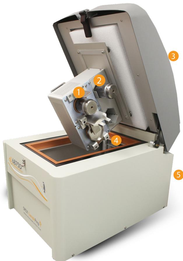
1. Dual grinding chambers accommodates a total of 200 grams of sample. (100 grams per chamber.)
