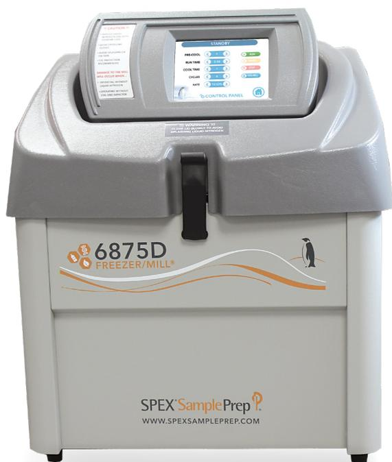
The 6875D Freezer/Mill® is a high-throughput, dual chamber, cryogenic grinder with a self-contained liquid nitrogen tub and insulated case. It chills samples in liquid nitrogen then pulverizes them with a magnetically driven impactor. It accommodates samples in the 0.1 gram to 200 gram range (100 per grinding chamber).
